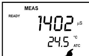
Figure 11 - ATC annunciator will light up when connected to temperature probe
